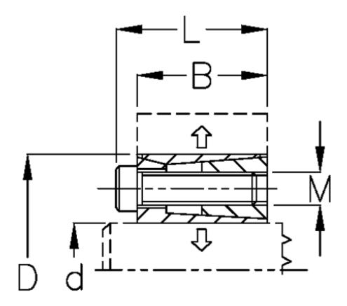
B mm = 18d mm = 32D mm = 54Fit tolerance = Aksel h8, Nav H8
